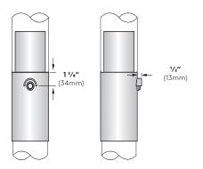
**Photo Cell Tenon (PCT)** - Button type photocell mounted in cast aluminum pole top tenon. Tenon has integral cast visor to prevent false start/stop cycle and can be oriented for optimum performance. Refer to luminaire spec sheet to determine if this option is applicable.
